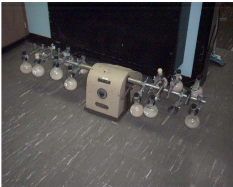
Figure 4. Photo of a batch experiment on the wrist shaker.
