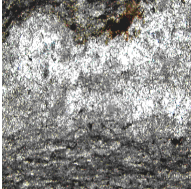
Figure 1. Petrographic image of Minnekahta Limestone (10x; image dimensions 1.5mm x 1.5 mm).
