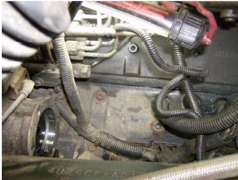
Photo #6: Engine block after hole has been drilled
