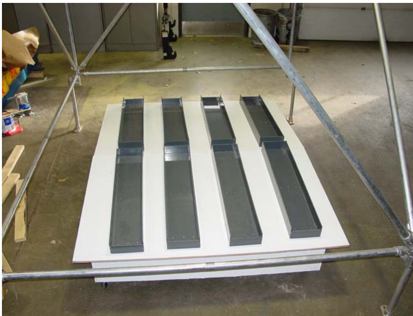
Figure 4. Runoff boxes used for indoor rainfall simulation.
