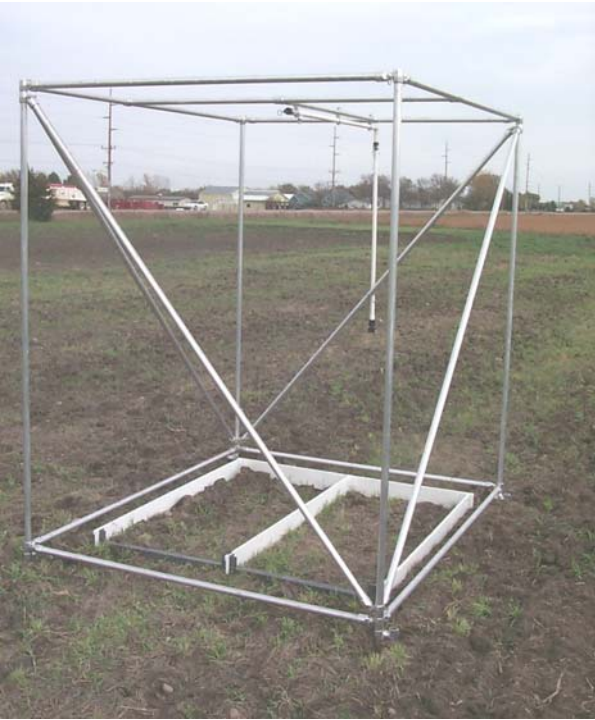
Figure 3. Rainfall simulator used for P runoff evaluations.
