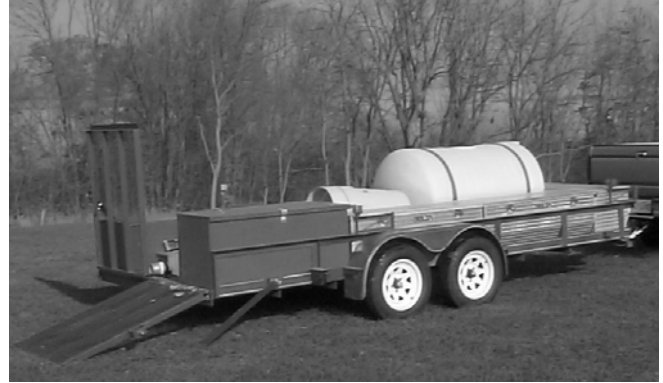
Figure 2. Goose-neck trailer with 1600-gal. capacity water tank. (Chem-tainer Industries, Inc. 361 Neptune Ave. West Babylon, NY 11704, 516-661-8300).
